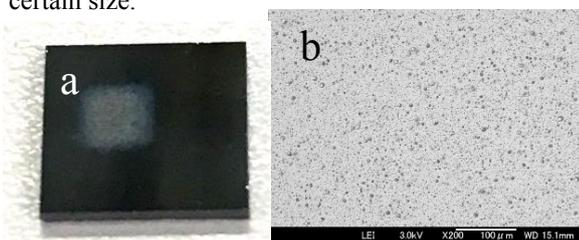
Fig. 1 (a) Photograph of aerosol sample collected on a Si substrate. (b) Low magnification SEM image of collected area.
