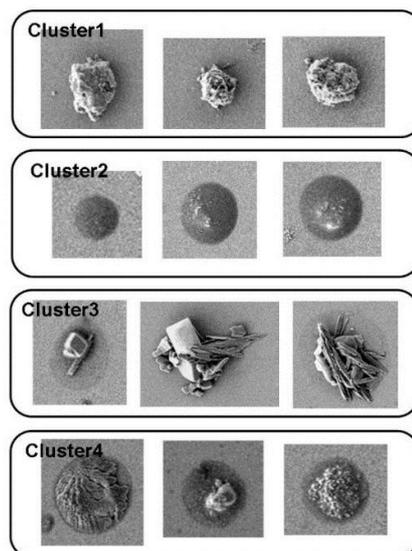
Fig. 3 SEM images of typical aerosol particles of each cluster.
