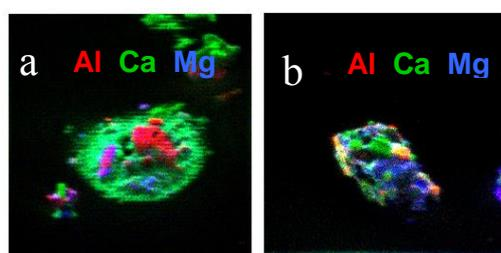
Fig. 2 Positive mode TOF-SIMS maps of main components in (a) dissolved yellow sand (chlorinated yellow sand), (b) dry yellow sand.
